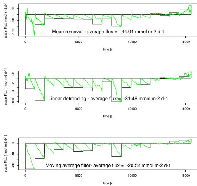
The large impact of non-stationarity is an important drawback for the application of aquatic eddy correlation techniques in such dynamic environments as estuaries and coasts. Preliminary results indicate that tidally averaged results are still reliable. However, we only have some empirical evidence, and it seems there is no theoretical guarantee that tidal averaging reduces the impact of non-stationarity effectively to zero. This requires further research.
